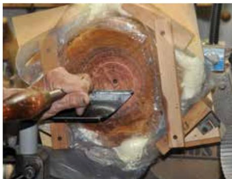
**Turning the inside without revolving tailstock centre support**
