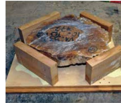
The battens glued in place to create the dam/wall around the work
