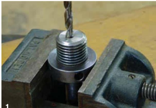
Drilling the first hole into the carving stand.
